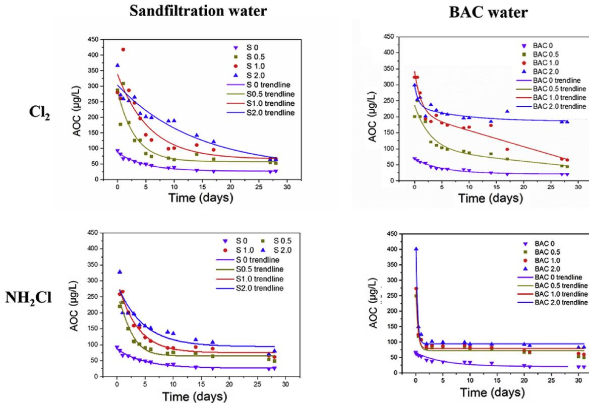
Fig. 6. Comparison of AOC variation of different water (sand filtration water and BAC water) with different dosages of disinfectant (chlorine and chloramine) during the 30-day bench test.
