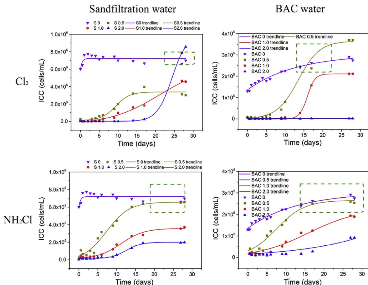
Fig. 7. Comparison of ICC variation of different water (sand filtration water and BAC water) with different dosages of disinfectant (chlorine or chloramine) for a 30-day bench test.
