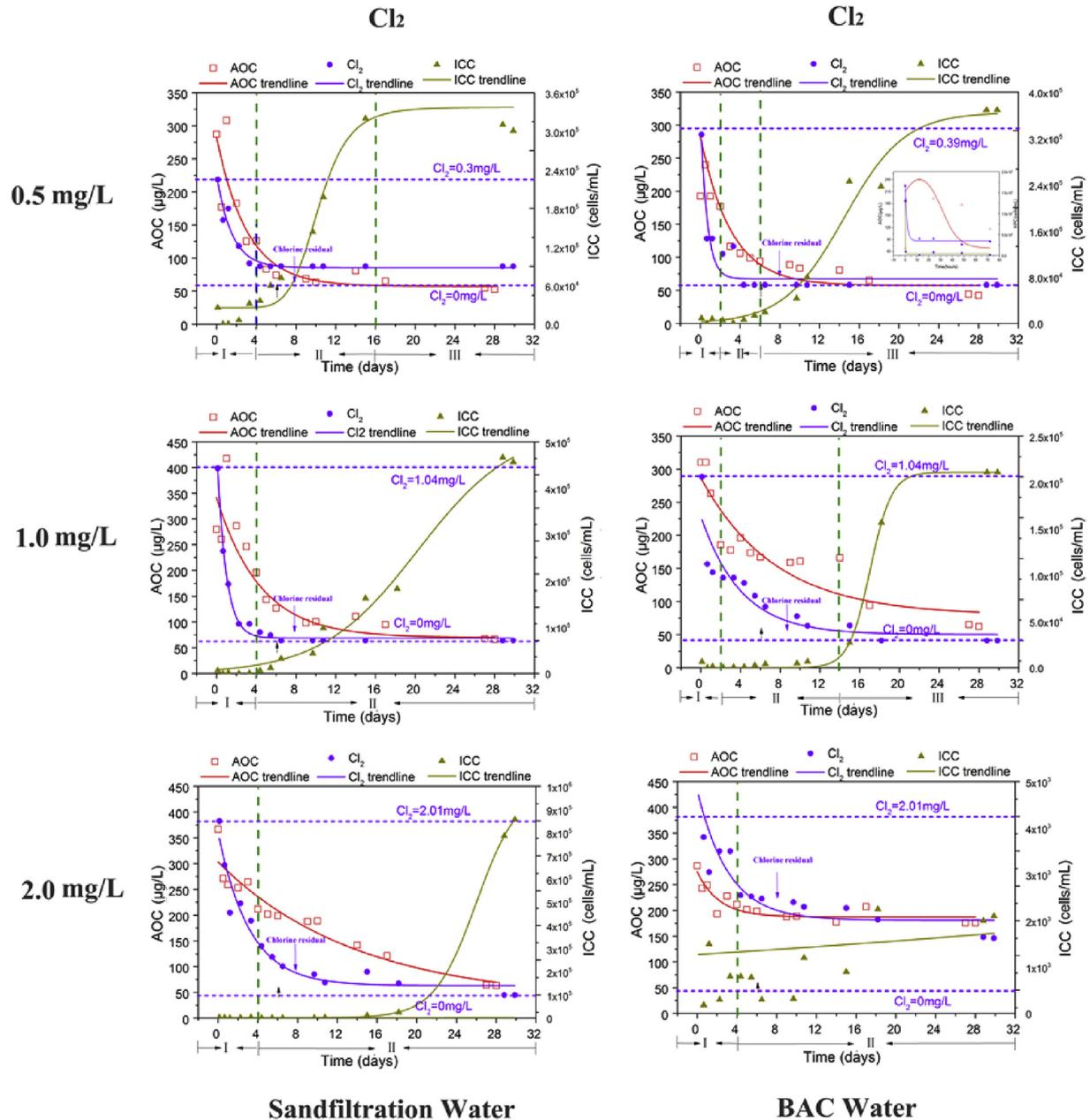
Fig. 4. Variation of biological stability of sand filtration water and BAC water with different amounts of chlorine and chloramine residuals in the bench test.
