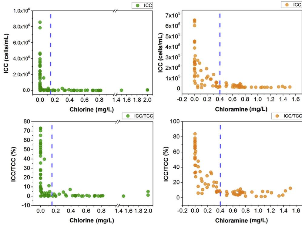
Fig. 5. Statistical analysis of orthogonal experiment results testing the effect of disinfectant concentrations on intact cells and the relative proportions of intact cells in chlorinated and chloraminated systems.
